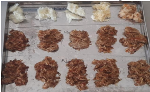
Fig 2: Extracted Cellulose fibres treated with different bleaching agents at varied concentrations showing comparative variation in their appearance
